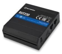
Small and reliable cellular router with 3G & WiFi. Equipped with Ethernet and I/O. RUT230 is perfect for challenging applications within energy, industry, smart city and IoT sectors.
